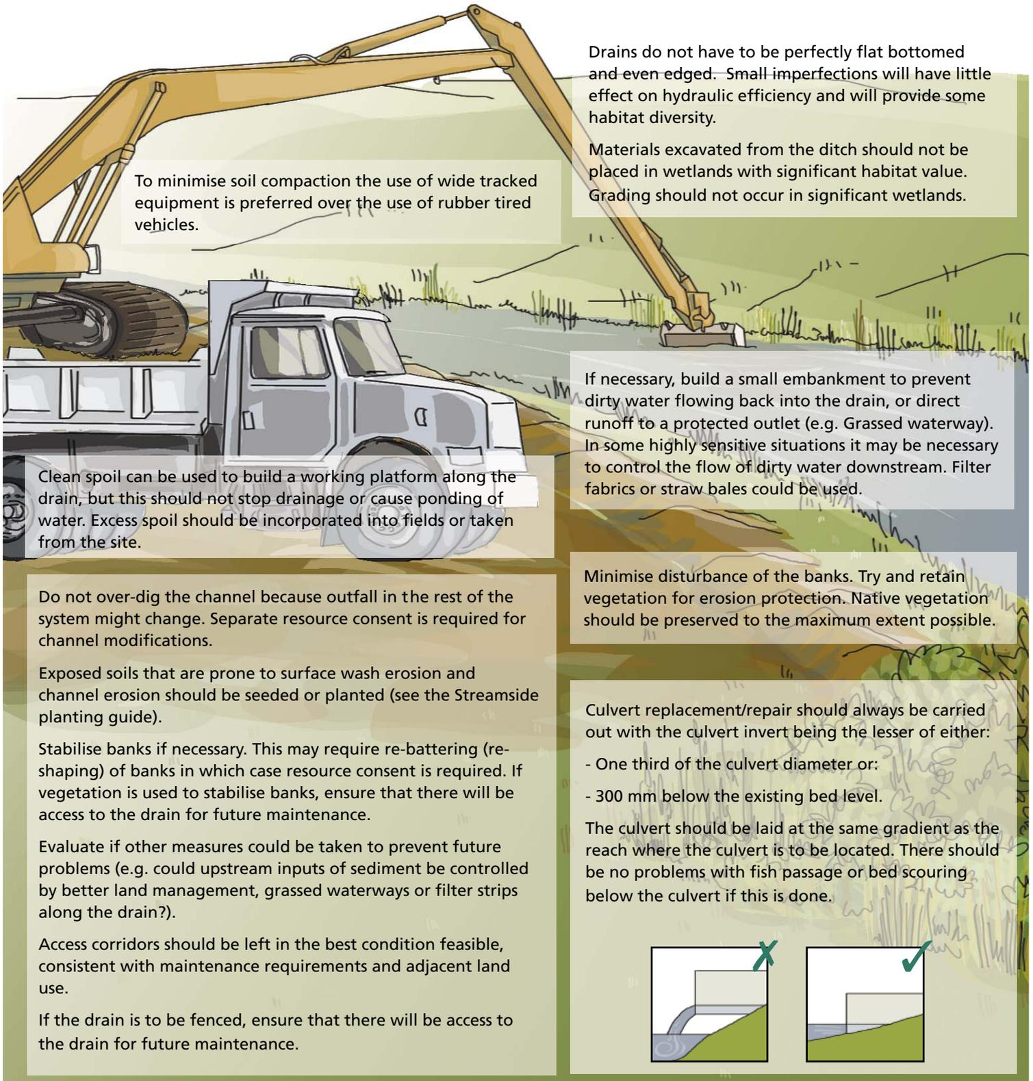
To minimise soil compaction the use of wide tracked equipment is preferred over the use of rubber tired vehicles.
