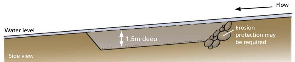
The upstream edge of the pit probably has to be stabilised with rock to prevent erosion. (If the bed erodes the trap will fill up with this material). Make sure that fish passage can still occur.
