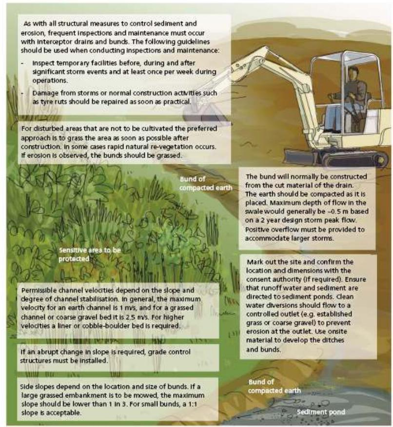
The bund will normally be constructed from the cut material of the drain. The earth should be compacted as it is placed. Maximum depth of flow in the swale would generally be -0.5 m based on a 2 year design storm peak flow. Positive overflow must be provided to accommodate larger storms.
